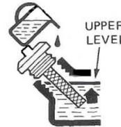
When the engine crankcase is full, the oil level should reach the lower lip of the oil filling opening as illustrated in Figure 2.
