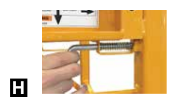
H Make sure that all four Lock Pins are secure and in LOCKED position.
