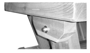
C. On the outside of the chair, secure Carriage Bolt (E) with Washer (D) and Locking Nut (C) with 11mm or 7/16 socket.
