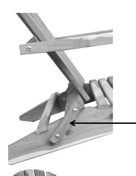
G. Be sure to rotate the Hinge Block once the Block is attached on both sides. Once rotated, tighten all bolts using an 11mm or 7/16 socket.
