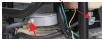
LP Gas Inlet (Figure B)
